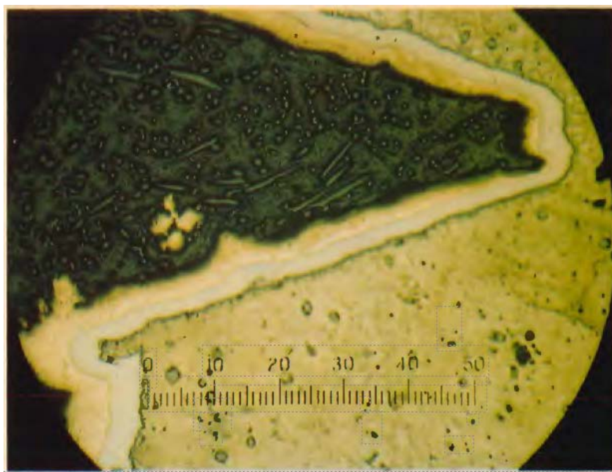
Fig. 3 — A 25 \mu\text{m} (1 mil) electroless nickel coating reproduces profile of internal threads on leaded steel part. Note nonuniformity of copper overplate. Picral. 100X.
