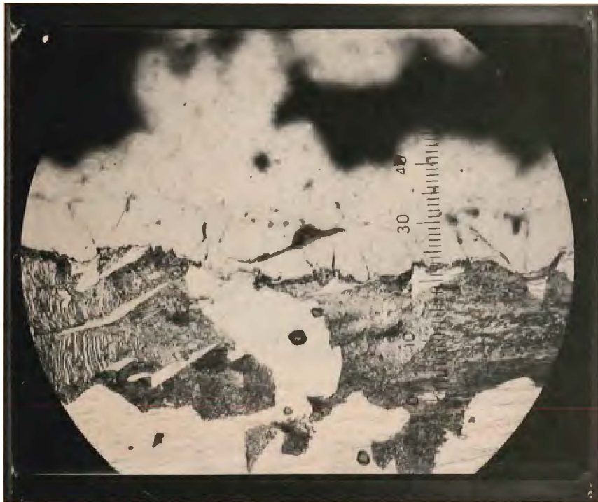
Fig. 2 — Typical low phosphorus (<10% P) electroless nickel deposit on AISI 4140 steel substrate. Coating thickness is 20 \mu\text{m} (0.8 mil). Cracks and pores are due to high stress level of deposit and co-deposited contaminants. Nital. 400X.
