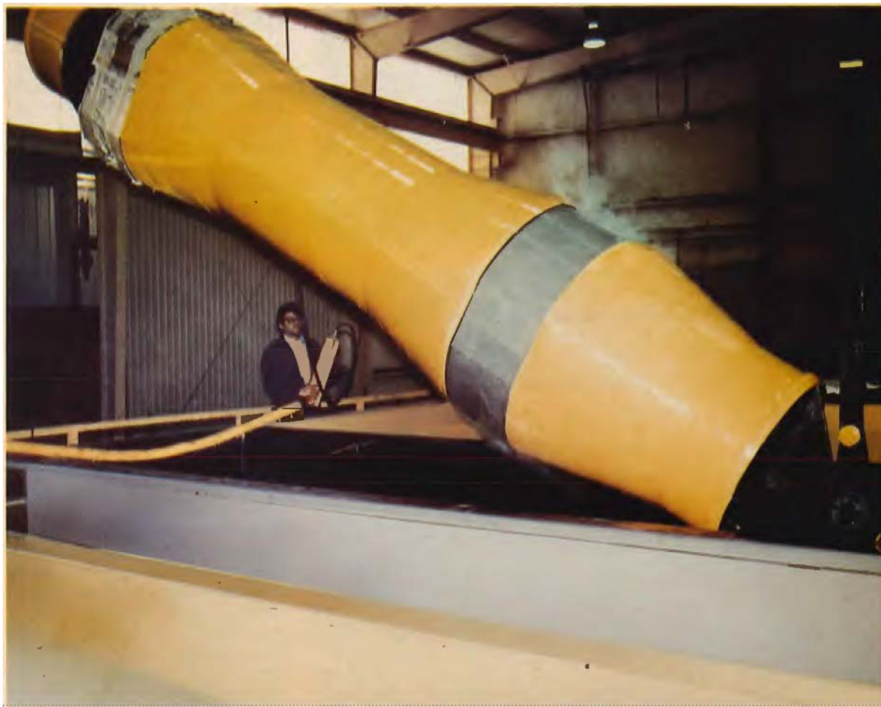
Fig. 4 — Bearing surfaces of 8200 kg (18 000 lb) shaft for turbogenerator are coated with 100 \mu\text{m} (4 mils) of electroless nickel to protect against vibration produced during startup and shutdown of equipment. (Courtesy Schumacher Co., Houston)
