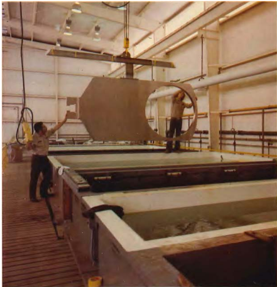
Gate for 1.2 m (48 in.) flow line gate valve was coated with 75 \mu\text{m} (3 mils) of electroless nickel for corrosion protection. (Courtesy Schumacher Co., Houston)
